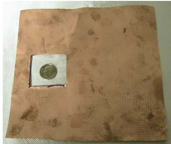
b) Damage to sensor with one 2.5 cm hole
