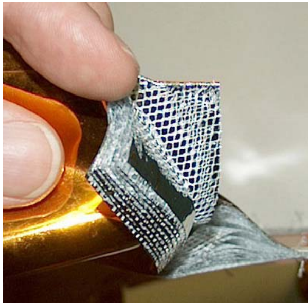
Figure 2. Multi-layer Insulation (MLI) construction
