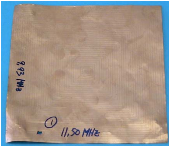
a) Damage to sensor with one 2 mm hole
