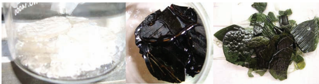
Figure 4. Low-temperature supporting electrolyte (left), with 25 wt. % iron oxide (center), and with 23 wt. % JSC-1 lunar simulant (right).
