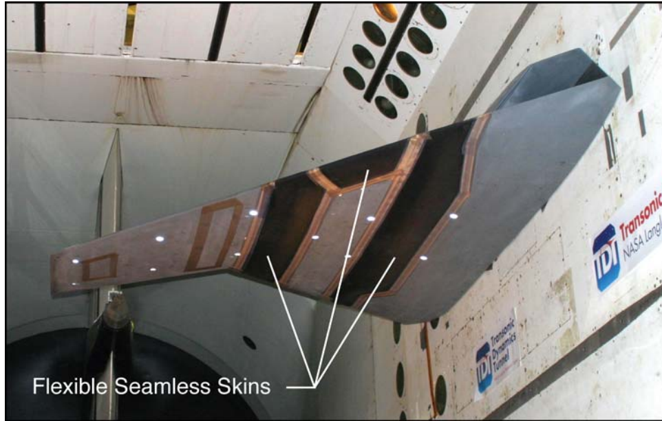
Figure 9. Lockheed Martin MAS Model Mounted in TDT
