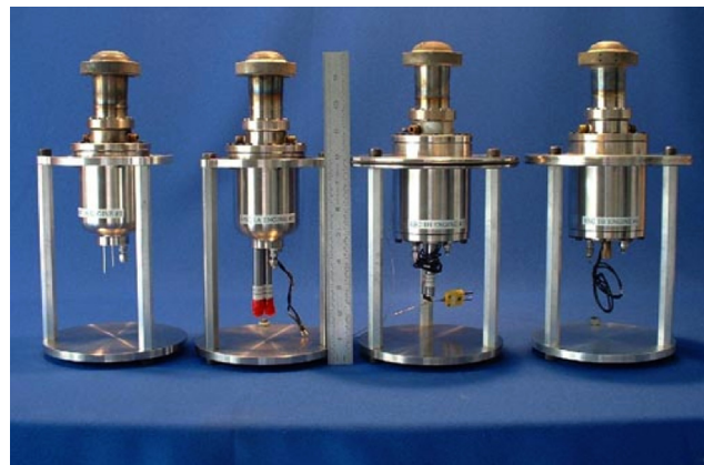
FIGURE 4.2 —Four ASC-1 engines built during Phase II.
