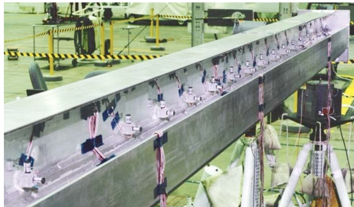
Figure 9. The Mock QS boom accelerometers.
