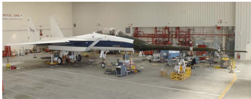
Figure 27. The GVT configuration of the mated QS with the F-15B airplane on soft supports.
