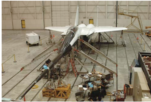
Figure 25. The GVT configuration of the mated QS with the F-15B airplane in constraints and on jacks.
