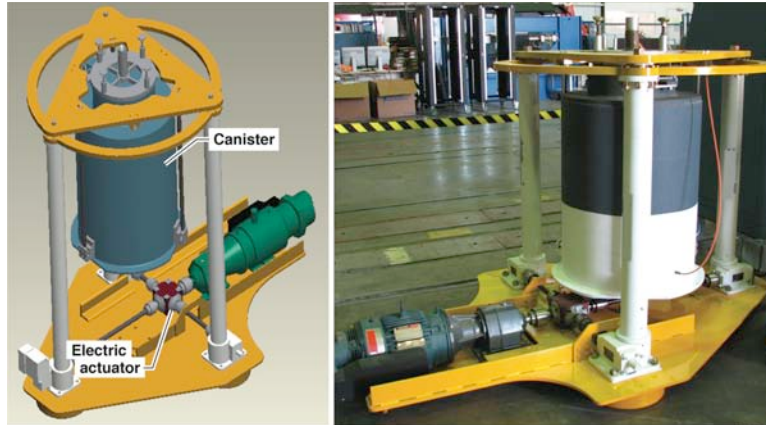
Figure 26. The NASA Dryden self-jacking soft support system.
