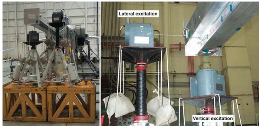
Figure 18. The shaker setup for the GVT of the Mated Mock QS with the F-15B airplane.
