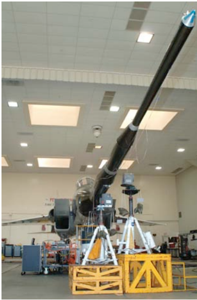
Figure 29. The shaker setup for the GVT of the mated QS with the F-15B airplane.
