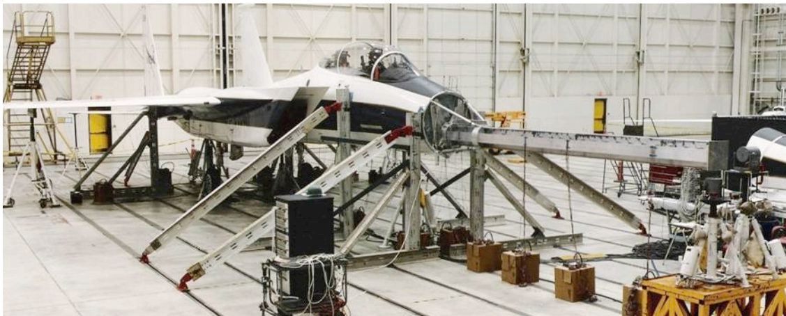
Figure 5. Mock QS boom ground vibration testing on the F-15B airplane.
