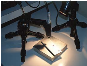
Fig. 3. Set-up for taking spectral measurements: optic pistol grip, quartz lamp, target.
