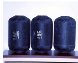
Figure 2. Filament wound resin and nanocomposite matrix tanks.
