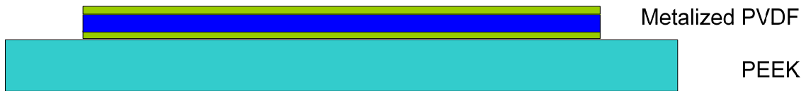
Figure E-6. Schematic of composite diaphragm
