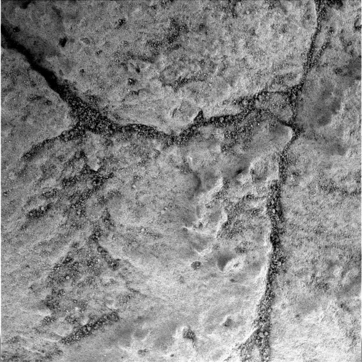
Figure S2: Microscopic Imager image of the lower unit of Home Plate, showing indistinct grain boundaries. Scale across the image is 3 cm. Microscopic Imager image 2M192682040.
