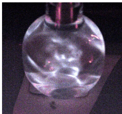
Figure 14.—Sonoluminescence created at NASA GRC (true color, contrast enhanced).
