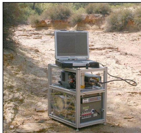
Figure 1. CheMin 4 instrument in Rio Tinto river bed with optional laptop computer for graphic user interface.
