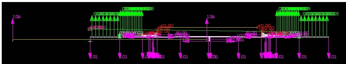
Figure 6: Boundary conditions on the patran insulated blackbody with the heat flux gage inserted 4mm from the center partition in the left cavity
