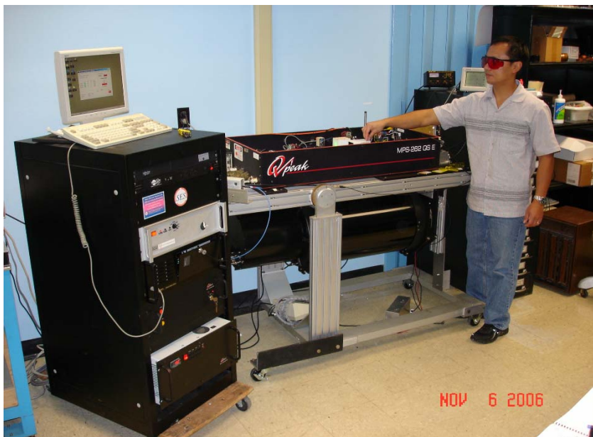
Figure 5: A picture of the compact DIAL lidar system taken within the lab.
