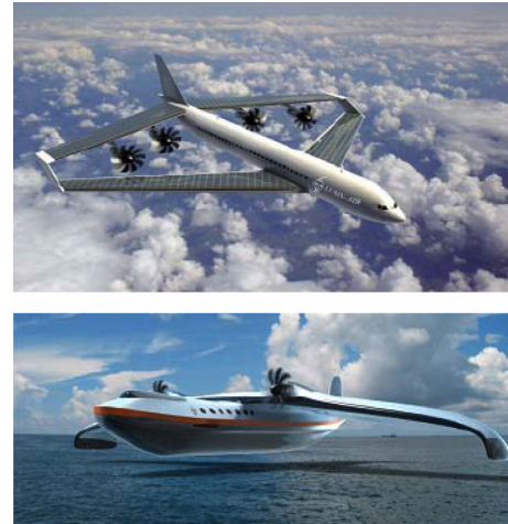
Figure 11.—Vision of future aircraft configurations powered by turboprops (lower and slower concepts). 37
