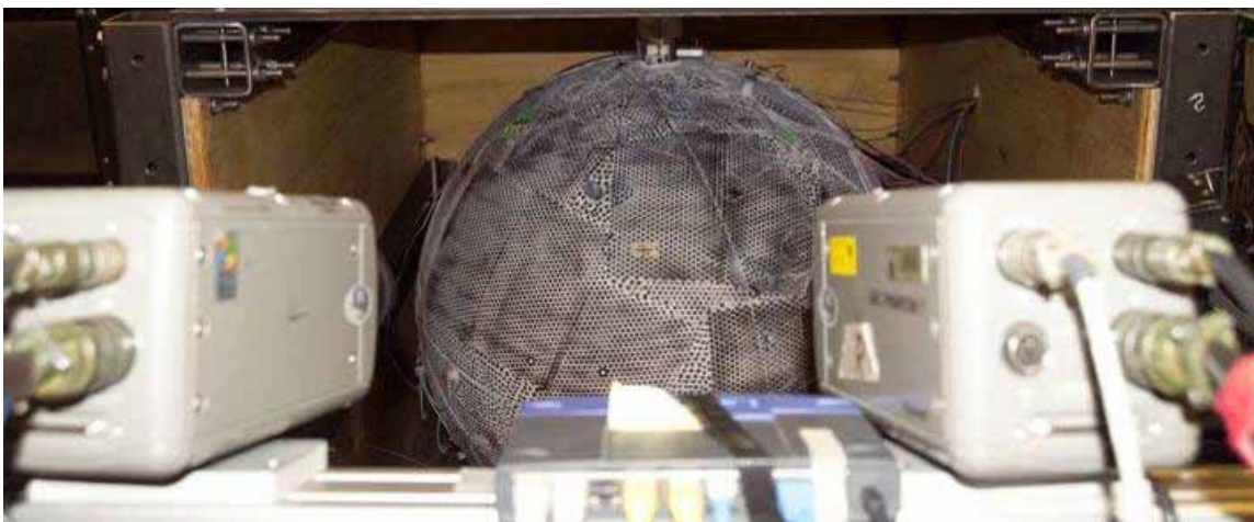
Figure 16. Digital image correlation camera view of COPV (Black dots sprayed over area of interest).
