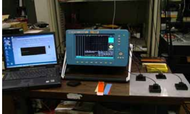
Figure 11. Eddy current inspection system for COPV composite thickness measurement
