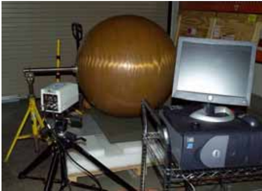
Figure 23. Heat soak thermography application to Kevlar COPV.
