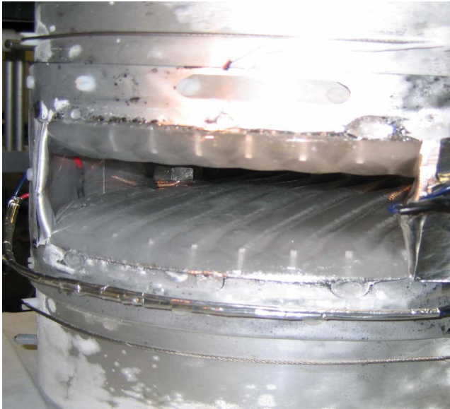
Figure 9. Large channel condenser image showing uniform ice deposition
