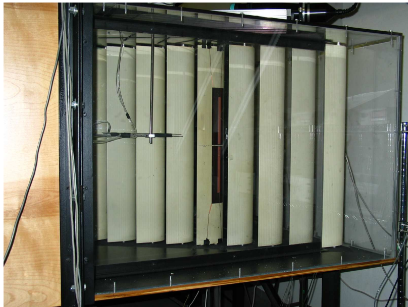
Figure 2.23. A commercially-made five-hole probe was used to measure the blade wake profiles.
