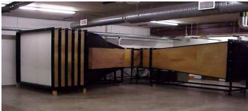
Figure 2.2. An open-loop wind tunnel was used in this work.
