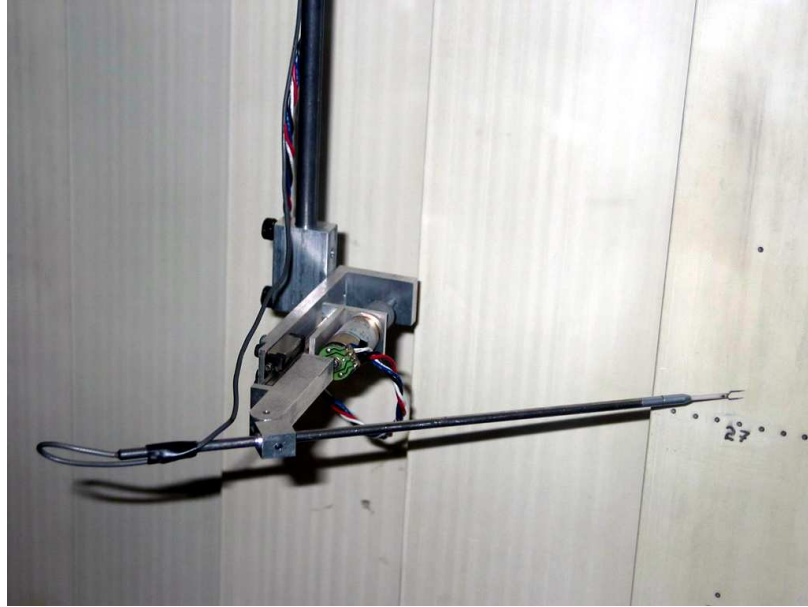
Figure 2.16. The hot-wire probe was mounted on a mini-traverse system which was aligned perpendicular to the local blade surface.
