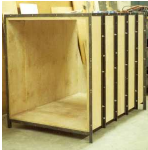
Figure 2.2. The screen boxes before final assembly.
