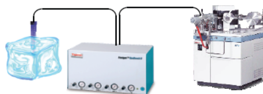
Figure 1. A cartoon of the experimental setup with a cooled vial containing the solution on the left, the Gas Bench II in the middle and the MAT 253 IRMS on the right.
