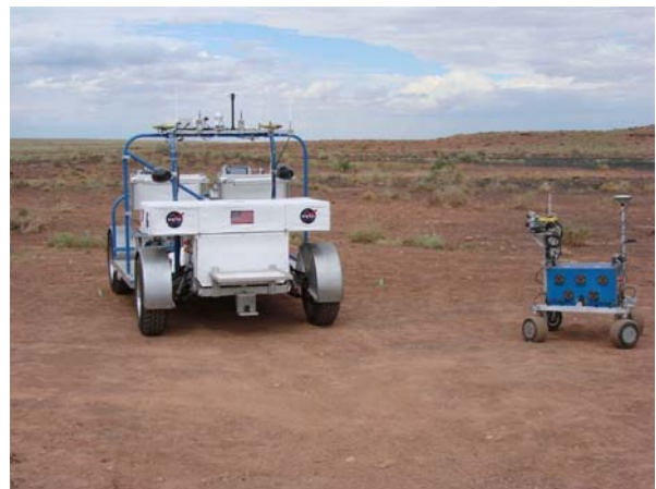
Figure 4: K-10 robot inspects SCOUT prior to SCOUT departing under supervised autonomy
