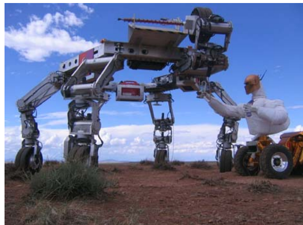
Figure 5: ATHLETE preparing to drill and Centaur removing a tether hook from ATHLETE
