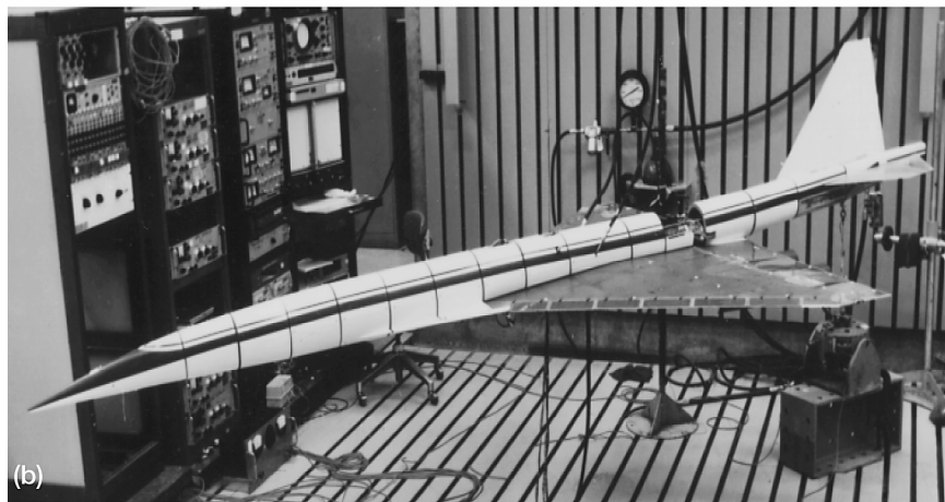
Figure 2.4.—(a) SST flutter model plate construction wing. (b) SST full flutter model assembly.
