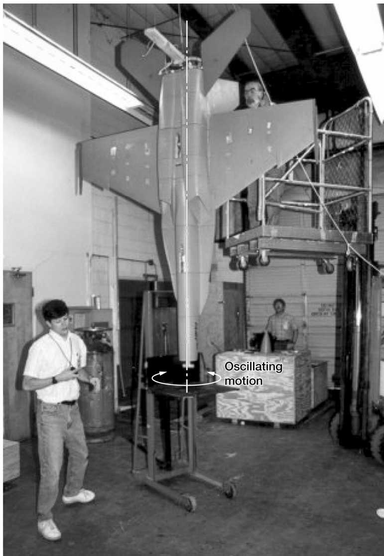
Figure 5.2.—(d) Full model roll inertia measurement using bifilar pendulum.
