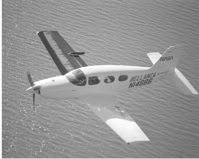
Figure 35.—Experimental aircraft for conducting laminar flow studies.
