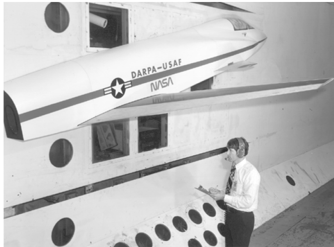
Figure 24.—Forward swept wing aeroelastic model mounted in TDT.
