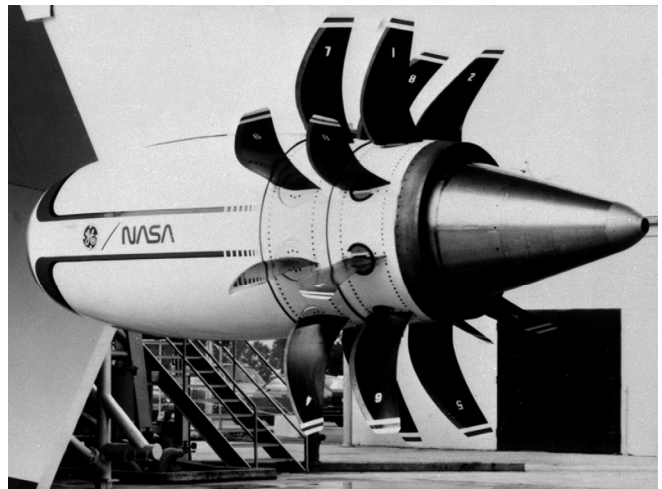
Figure 2.—Counterrotating propfan configuration known as counterrotating unducted fan.
