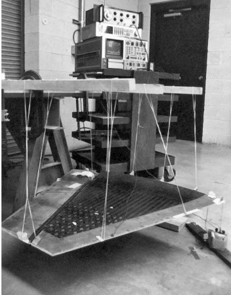
Figure 5.3.—(b) Component suspended to simulate free-free condition.
