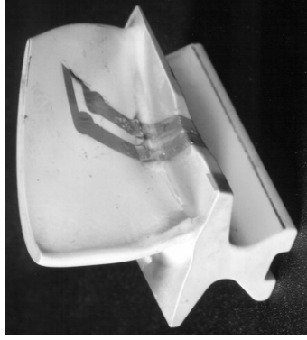
PdCr strain sensor to T=1000°C
