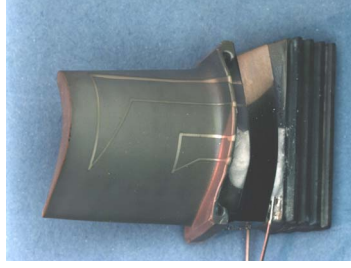
Pt- Pt/Rh temperature sensor to T=1200°C
