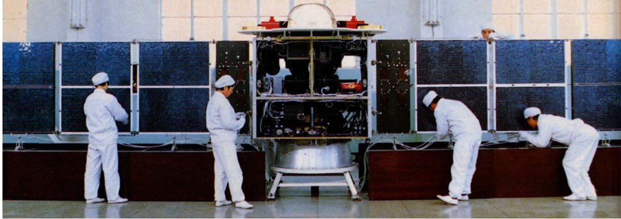
Fig. 1. A Fengyun-1 satellite in final assembly. The vehicle is shown in an inverted position; the sensors at the “top” point toward the Earth.
