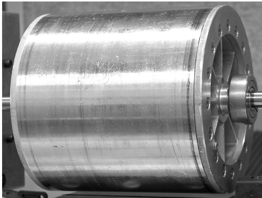
Figure 7.—Radial Halbach magnetic bearing test model rotor.
