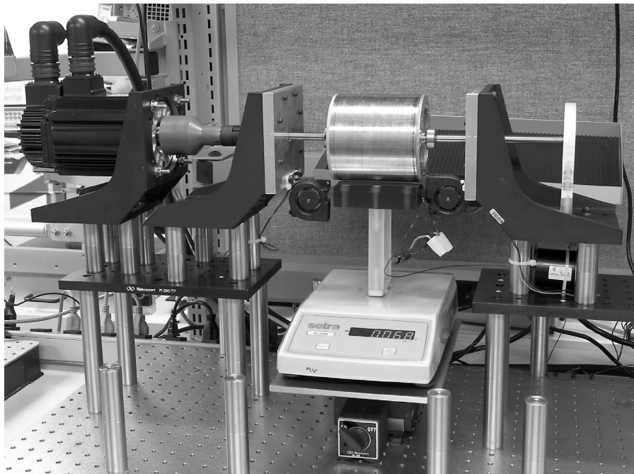
Figure 3.—Four inch radial Halbach magnetic bearing test model.
