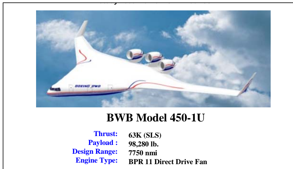
Figure 1. Baseline Blended Wing-Body trijet configuration used for this study.
