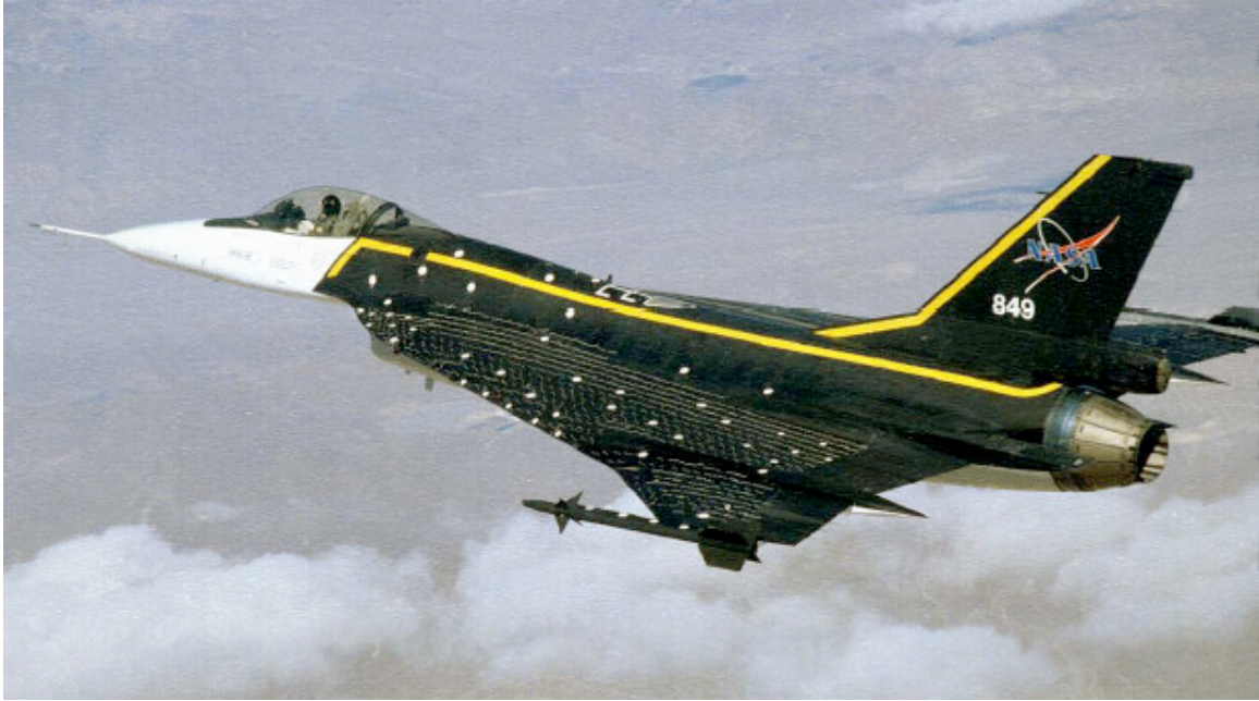
Figure 1. Missiles, tufts, modified flow-visualization paint scheme, and video targets on airplane at Dryden Flight Research Center (NASA Photo EC96-43508-2) 1 .
