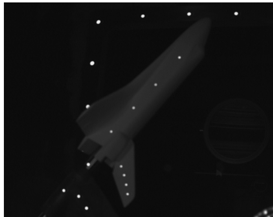
(b. IR illuminated targets for AoA tracking
