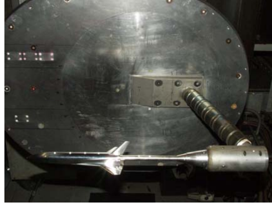
(b. Model injection system – 31-Inch Mach 10 Tunnel
