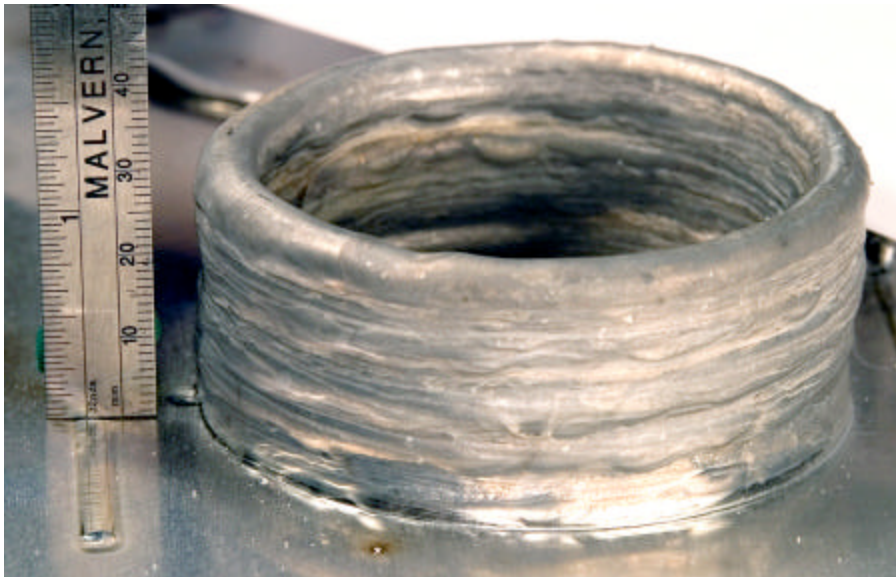
Figure 12. 30 mm tall cylinder built over two flights.
