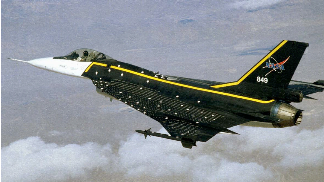
Figure 1. F-16XL-1 aircraft with missiles, tufts, modified flow-visualization paint scheme, and video targets at NASA Dryden Flight Research Center (NASA Photo EC96-43508-2).
