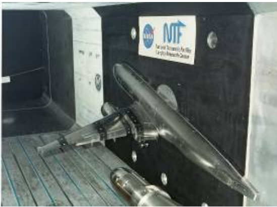
Figure-2. 777 Model in the NTF Test Section
