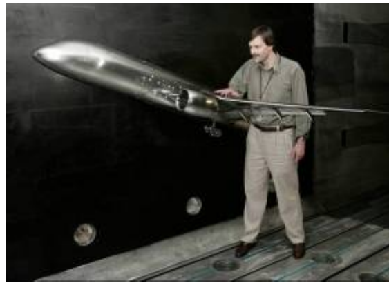
Figure-3. 787 Model in the NTF Test Section
