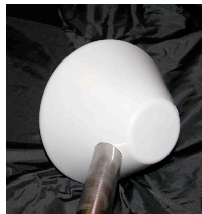
Figure 10. 3.03%-scale CEV model with powder coating.
