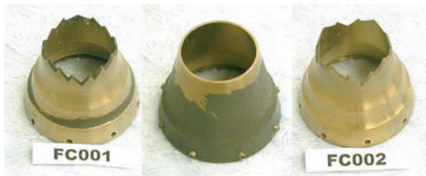
Figure 1.—The three nozzles presented in this paper are FCC001 (left), SMC000 baseline (middle), and FCC002 (right). FCC001 has three primary chevrons with smaller chevrons cut into the edges and FCC002 has four primary chevrons also with small chevrons cut into the edges.
