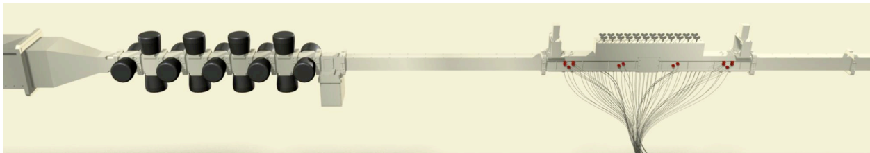
Figure 7. Sketch of NASA Grazing Flow Impedance Tube (GFIT) with test window moved downstream
