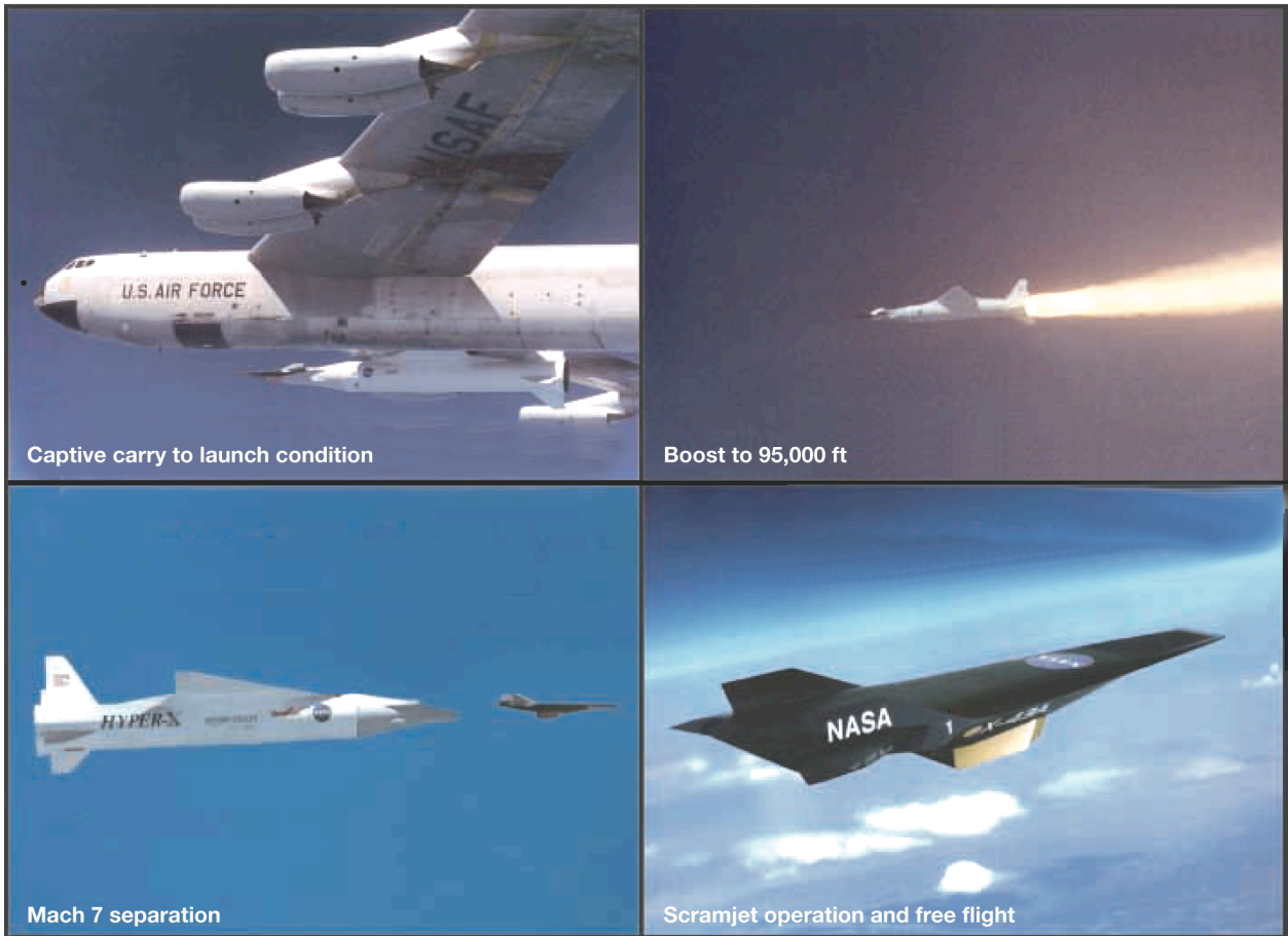
Figure 1. The four flight phases of the X-43A vehicle.
