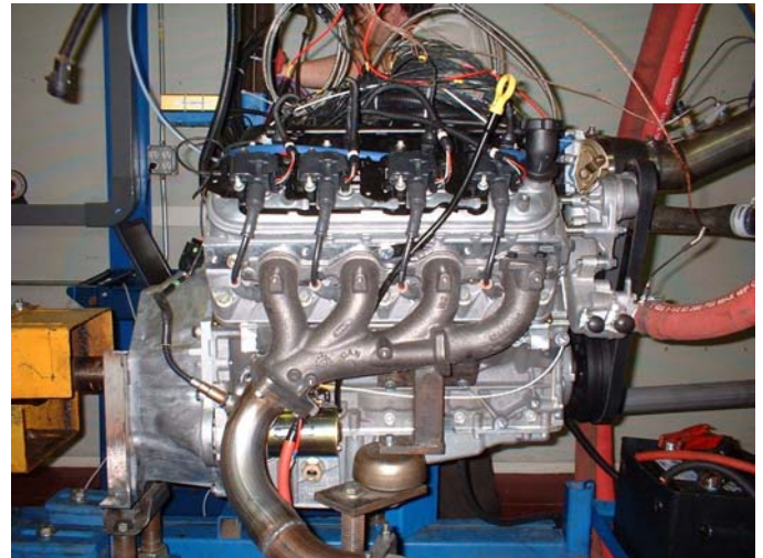
Figure 33 – Chevrolet LS-1 Engine Dynamometer Test
