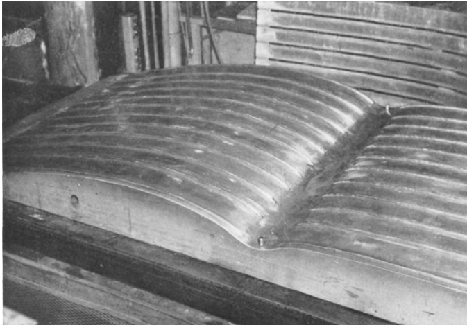
Figure 26 – Republic RC3 Seabee Production Wing Skin Press Die
