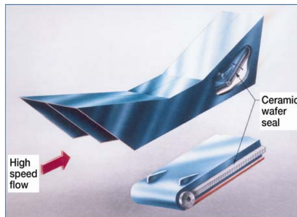
Figure 2. NASP engine panel edge seals designed to seal the gaps between movable ramps and adjacent engine sidewalls.
