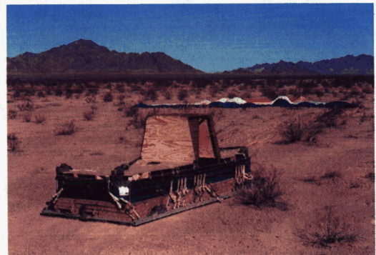
Figure 18. Platform configuration for backup parachute drop tests.
