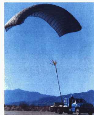
Figure 6. Truck tow test of 750 sq ft parafoil
