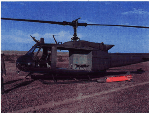
Figure 11. Medium DTV positioned on ground by Huey in preparation for drop test (DTV-10).
