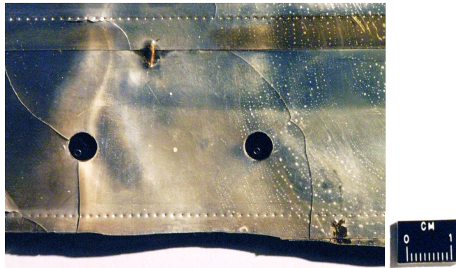
Figure 5. Close-up of the solar facing side of the SADA MLI showing through-thickness cracks and discolored regions.
