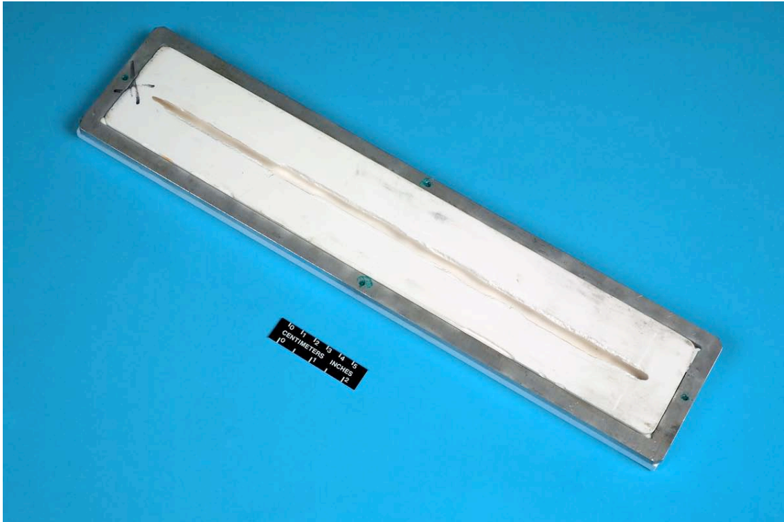
Figure 12. Lower side of ceramic model with attached aluminum mounting plate.
