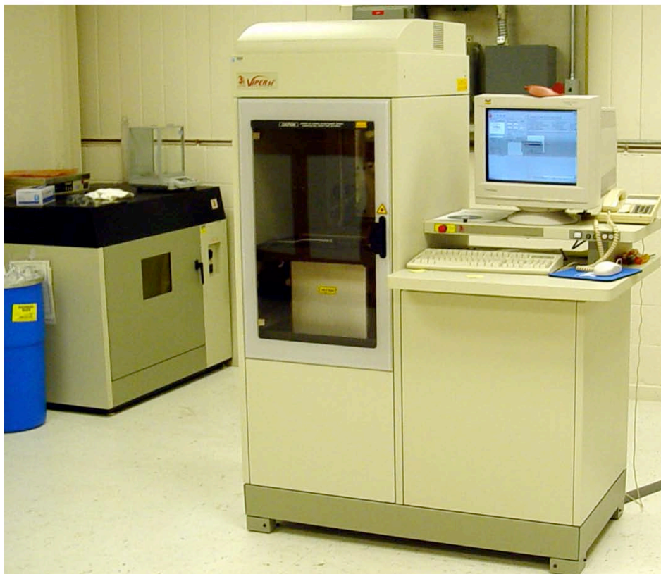
Figure 2. Rapid prototyping stereolithography systems used to build model patterns: top) SLA 7000 and bottom) Post Cure Apparatus and Viper SLA machine.
