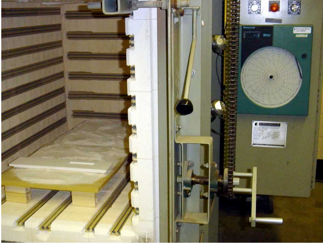
Figure 8. Sintering of cast ceramic model in electric fired kiln to 2150°F.
