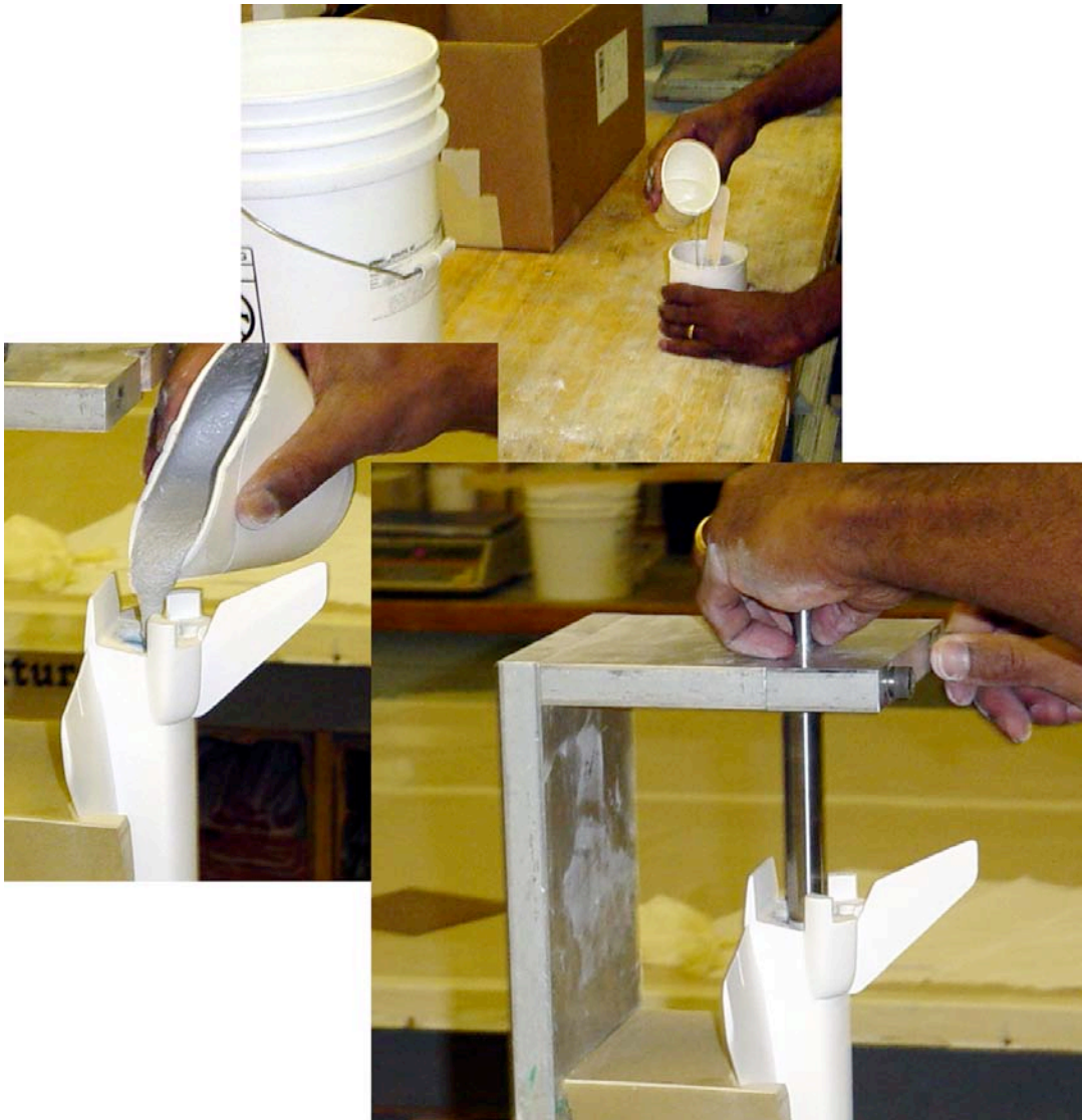
Figure 23. – Mixing, pouring and positioning hydraulic setting backfill material.
