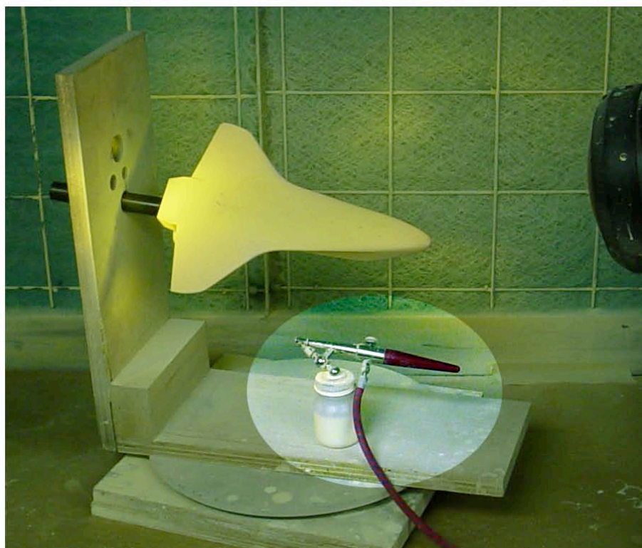
Figure 28. Spray booth and Passche Type H #5 air brush for phosphor coating.
