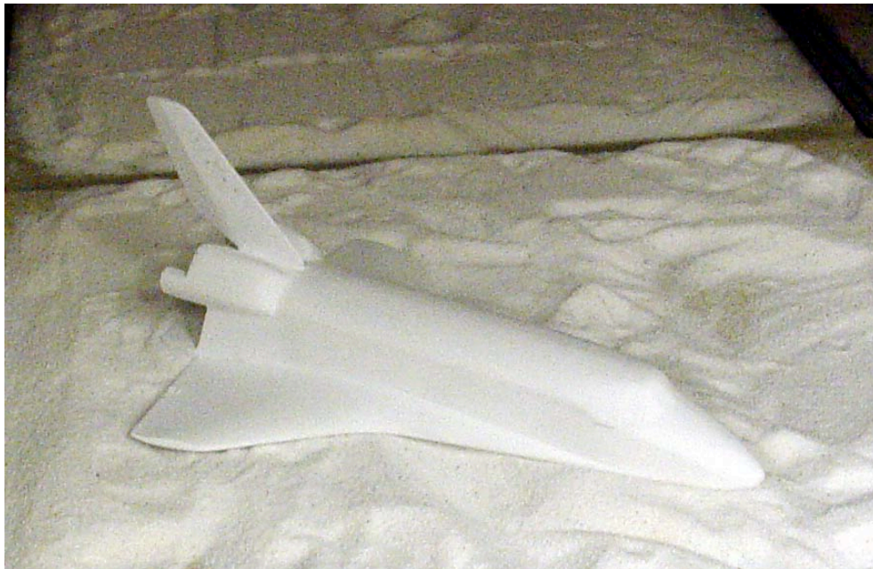
Figure 20. Sintered ceramic test model.
