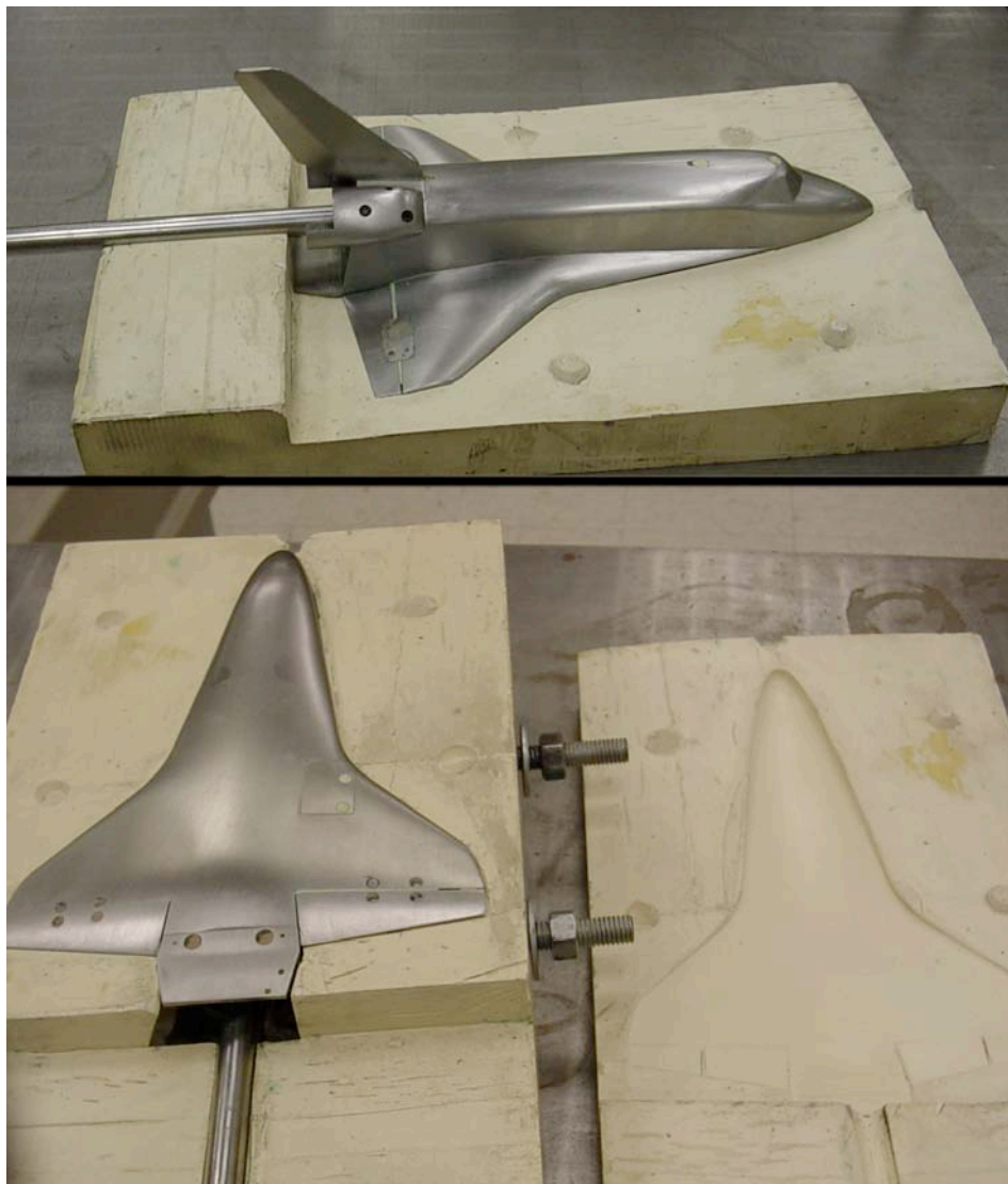
Figure 2. Top and bottom views of machined stainless steel aerodynamic test model/casting pattern and cast formed wax injection mold.
