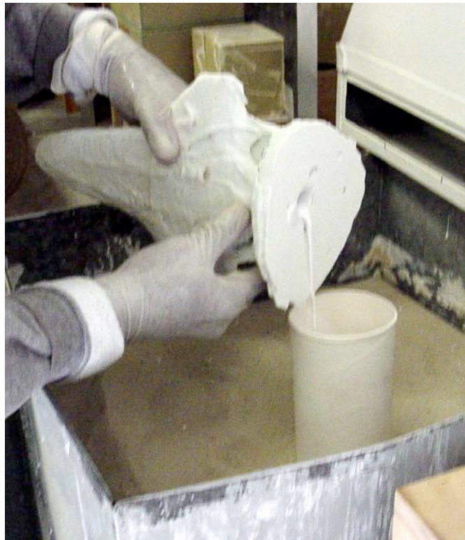
Figure 15. Removing ceramic slip from model center after 3/16 inch wall is formed.
