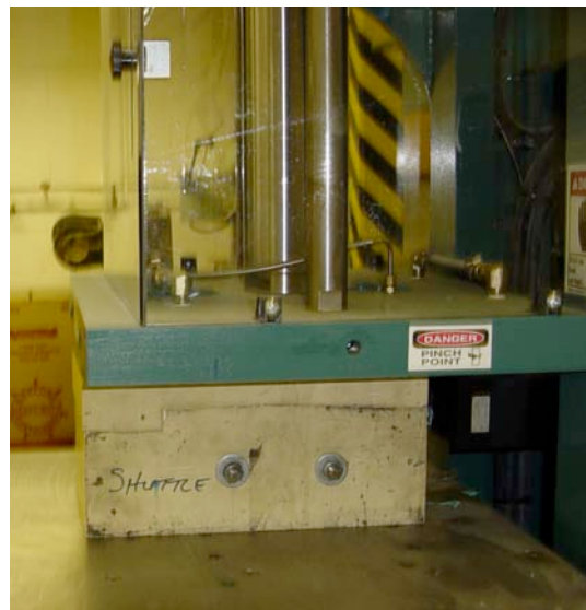
Figure 5. Injection of wax into wax injection mold.
