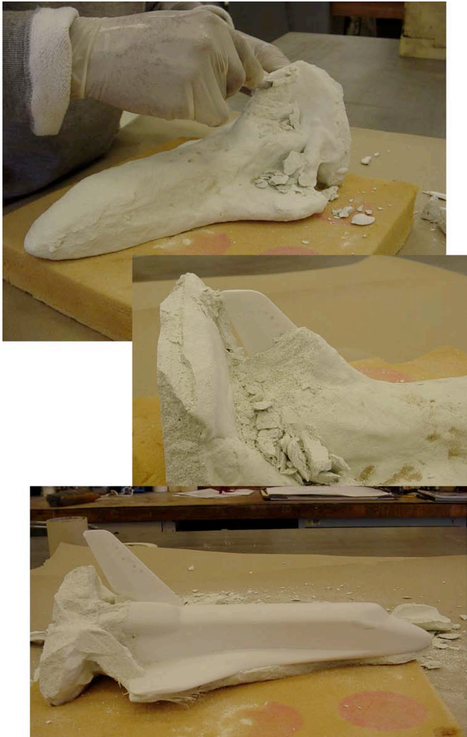
Figure 16. "Green" cast ceramic model being removed from shell mold.
