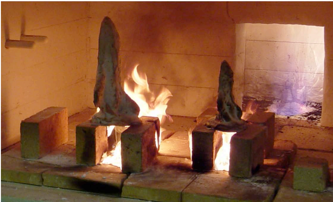
Figure 13. Removal of pattern from shell mold in wax “burn-out” gas oven.
