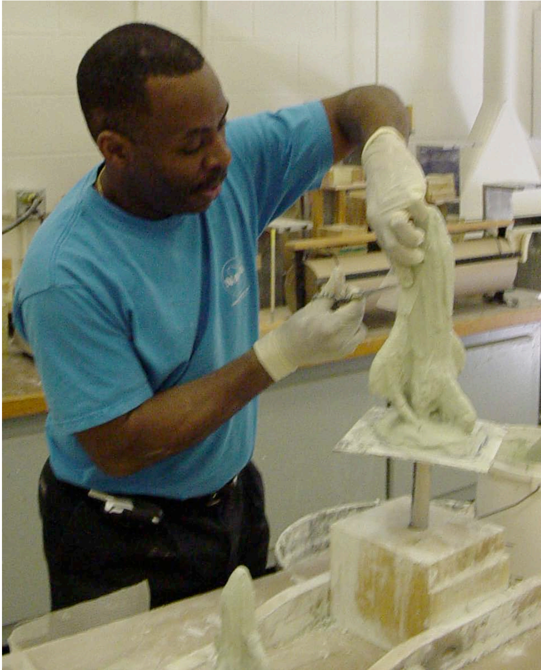
Figure 12. Reinforcement of shell mold with fiberglass cloth between fourth and final coat.
