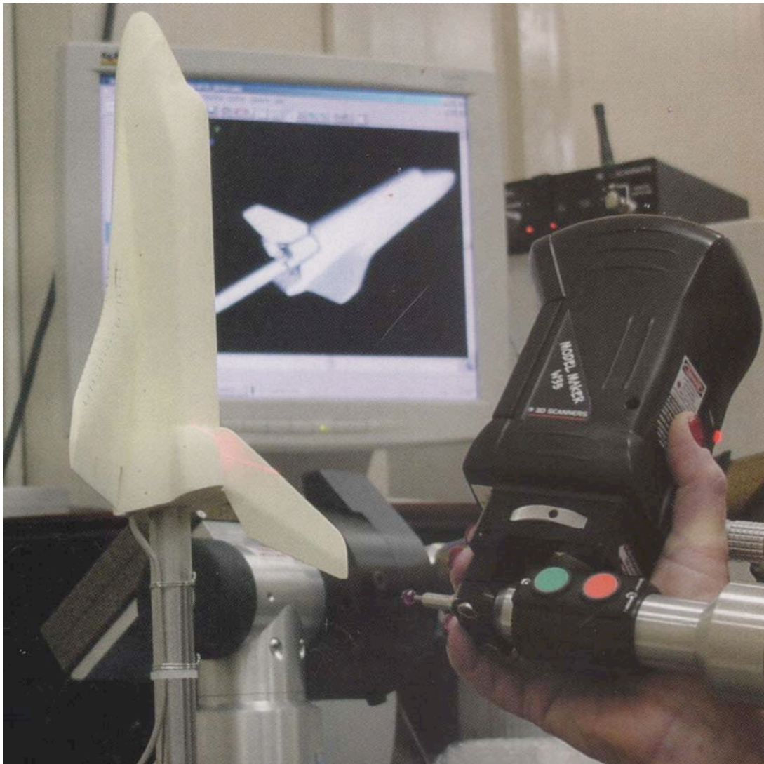
Figure 24. Portable laser scanner used for capturing pattern, mold and model surface geometries.
