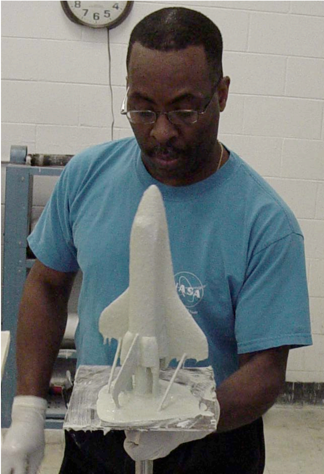
Figure 11. Completed first application of slip-casting investment shell mold to wax pattern.
