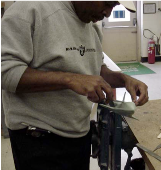
Figure 7. Trimming and cleaning of wax pattern.
