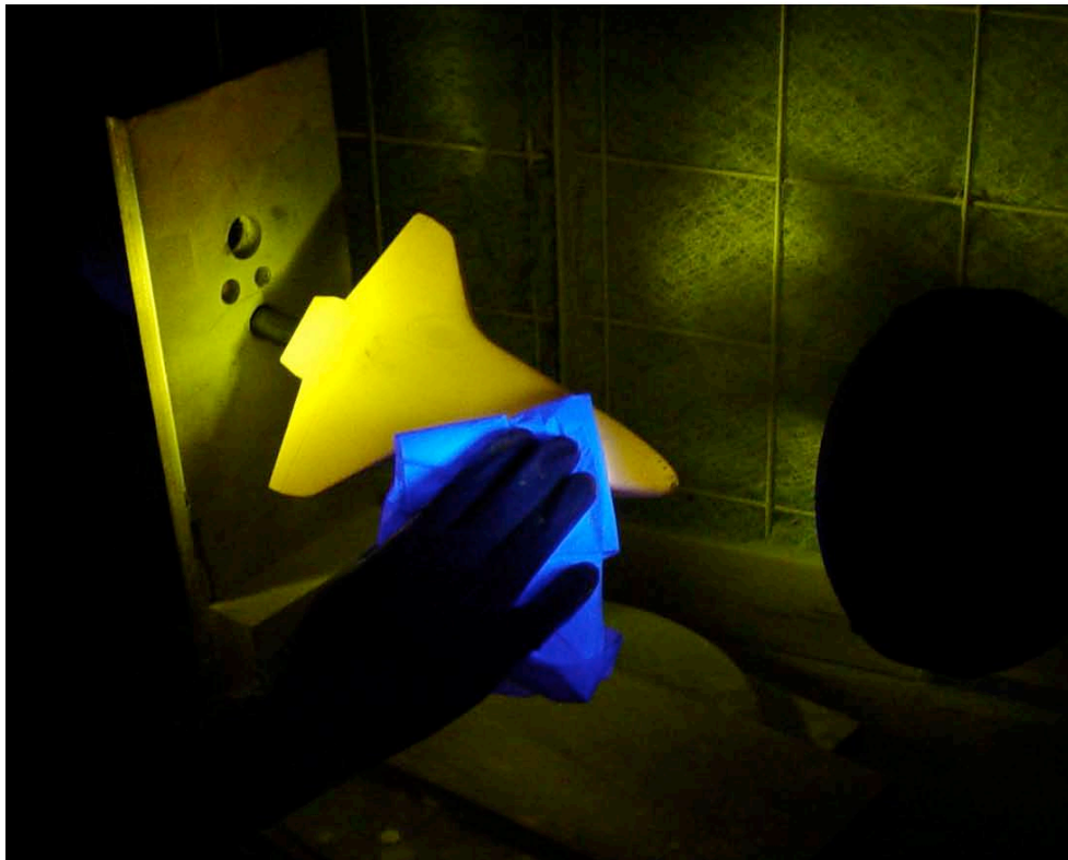
Figure 29. Spray coating and wiping excess phosphor coating.
