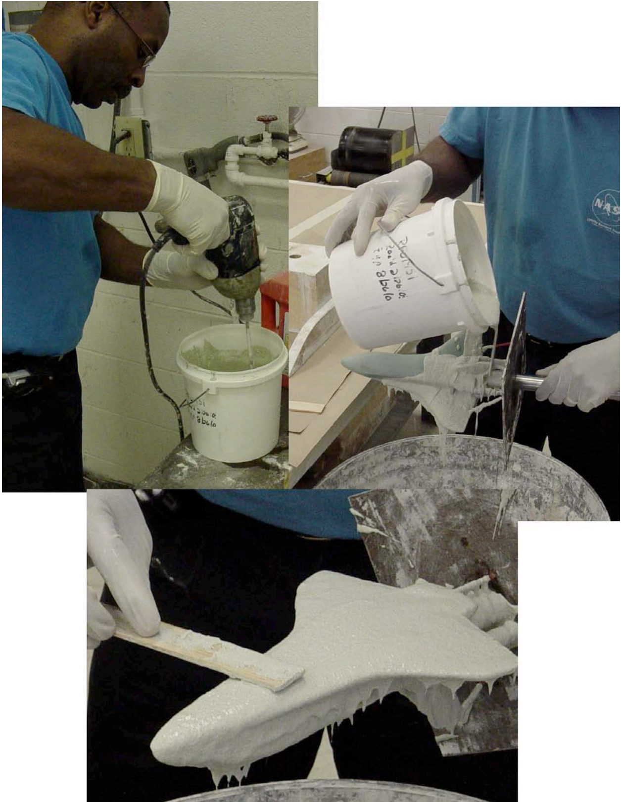
Figure 10. Application of slip-casting investment shell mold to wax pattern using a “buttering” method.
