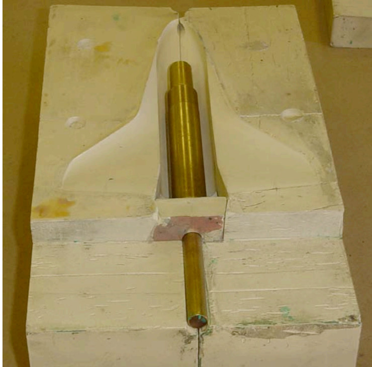
Figure 3. Two-part wax injection mold top section with aft insert piece and internal shaped brass core mandrel
