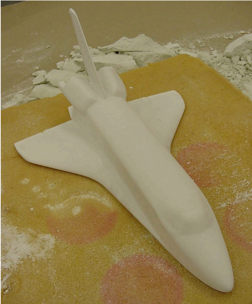
Figure 17. "Green" cast ceramic model "as cast."
