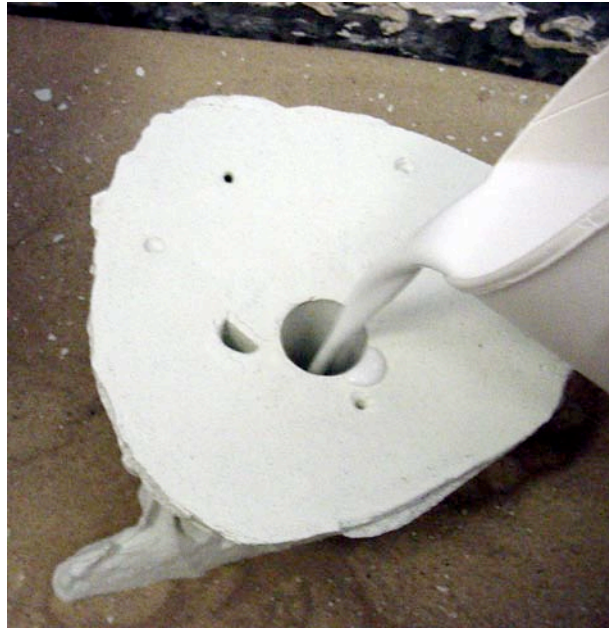
Figure 14. Adding ceramic slip material into investment shell mold.
