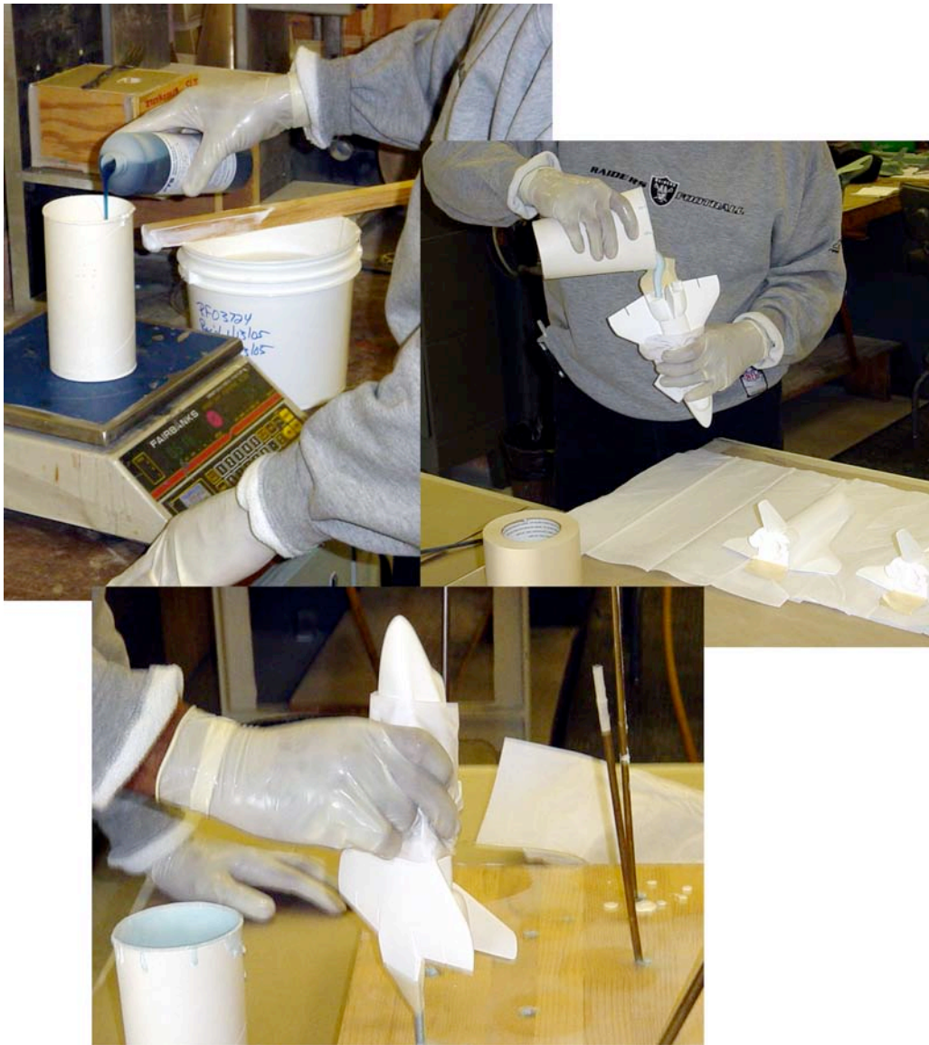
Figure 22. Mixing, pouring and draining GI-1000 Silicone liner to/from model cavity.
