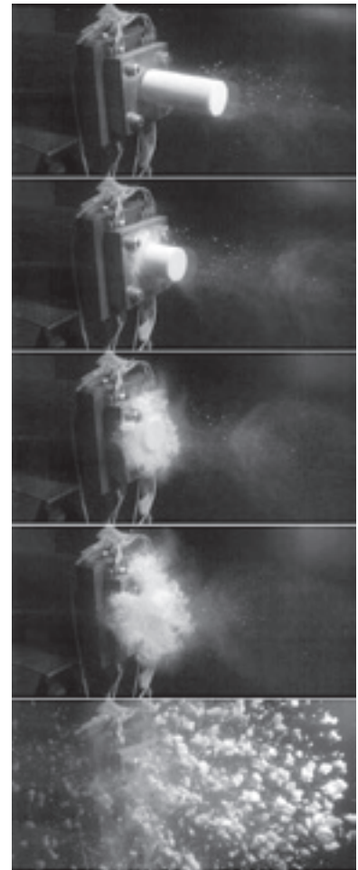
High-speed digital photography captures the behavior of external tank foam undergoing an impact event.
