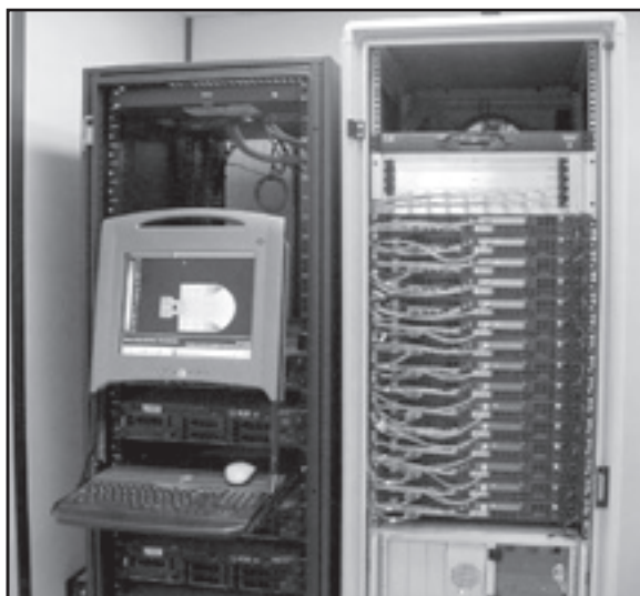
Parallel computer cluster for high-speed processing of complex-geometry Stirling simulations.
