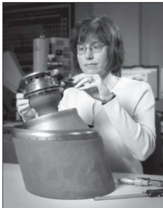
RCS thruster being examined optically for cracking in the relief radius.
