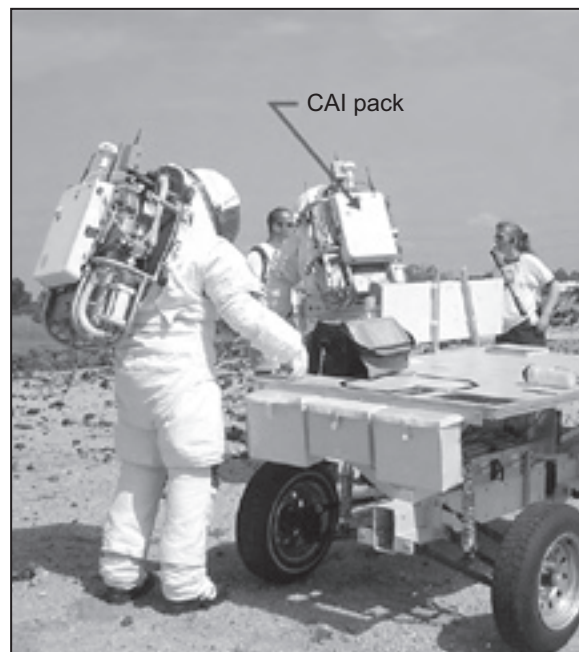
Two CAI packs mounted on each of the advance spacesuits during dry run testing at Johnson.
