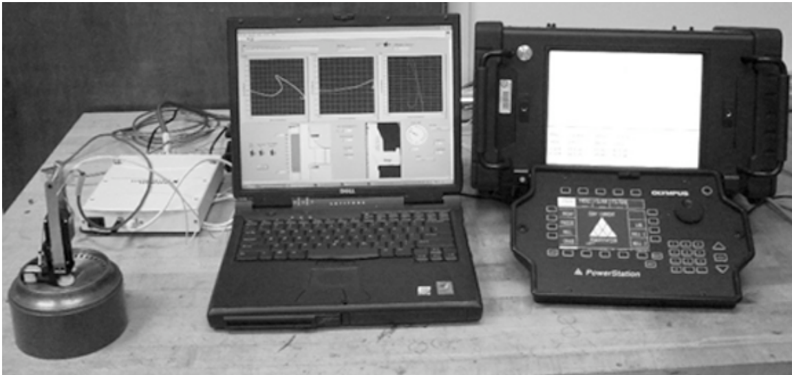
Figure 3. Complete eddy current PRCS thruster inspection system.
