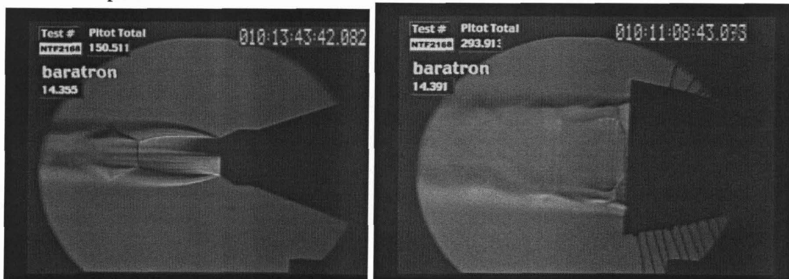
Figure 16. Schlieren Images of Stratford and Bell Nozzle Plumes (Flow Right to Left).
