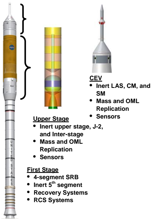
Figure 10. Components of the Ares I-1 development flight test vehicle.
