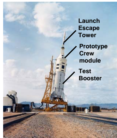
Figure 6. Apollo Launch Escape System (LES) testing.
