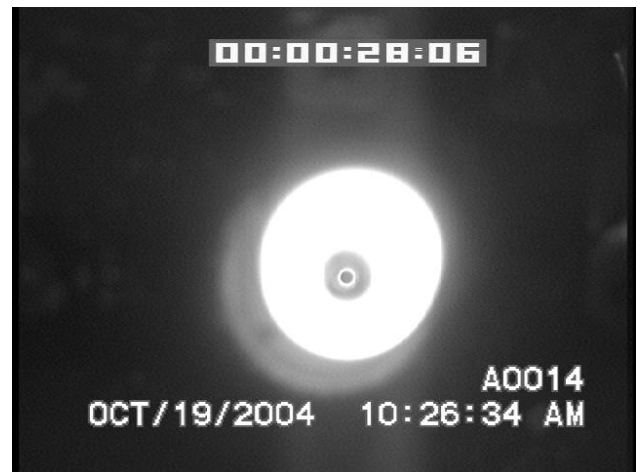
Figure 2 Top view Black\White Video Still after 5.0 seconds for same flame in Figure 1 showing open tip.
