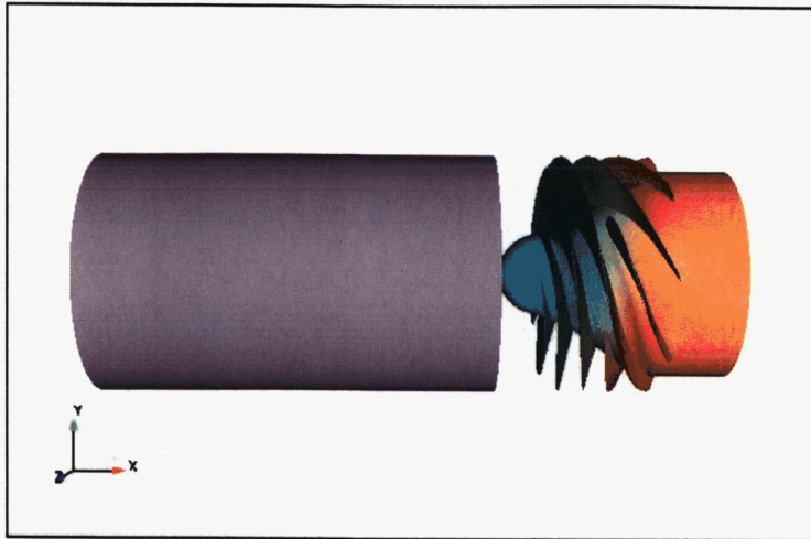
Figure 19. Perspective view of flow model for elliptical and eccentric tip clearance study.
