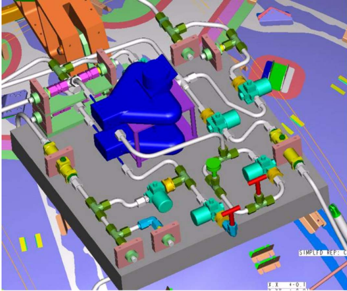
Figure 4.—CTB control panel.
