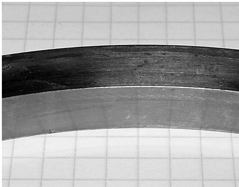
Figure 3.—Annular seal made of Inconel 625. Note, each grid square is 6.35 mm.
