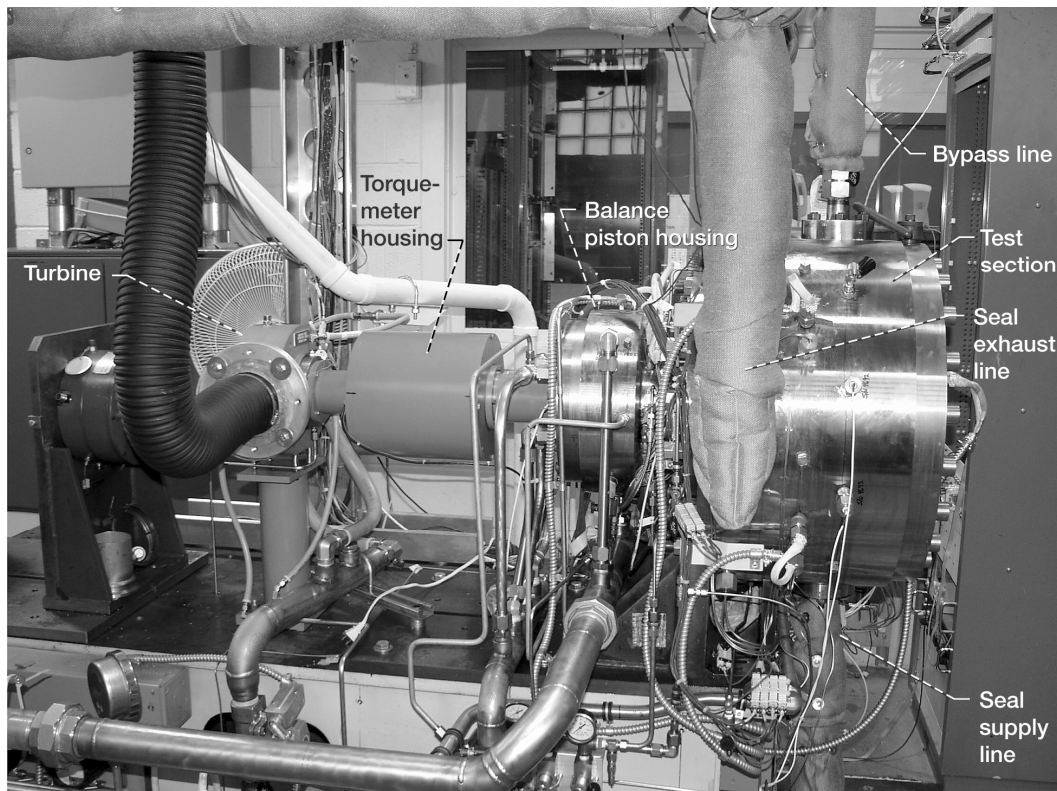
Figure 1.—High-temperature, high-speed turbine seal rig.
