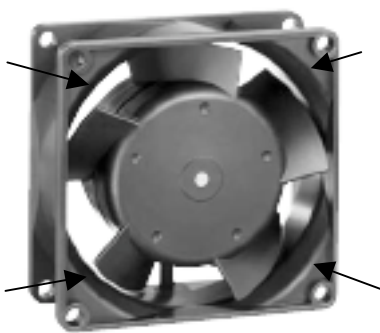
Figure 1.—Front view of test fan. Arrows show inlet regions where the rotor tip is uncovered.
